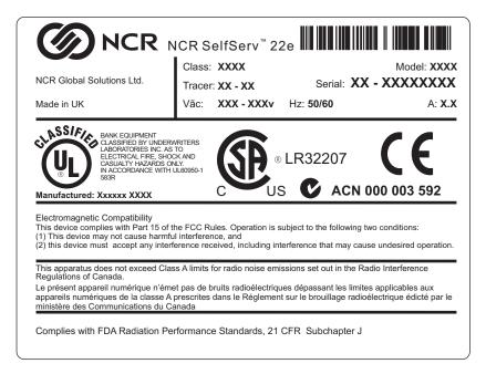
The product is identified by the class, and a 4 digit model number. The serial number is unique to each ATM. The tracer number is used to identify where the ATM was built.
